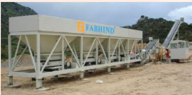
Wet Mix Macadam Plant
