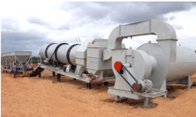
Drum Mix Plant
