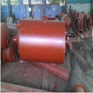
Water Seal Tank
